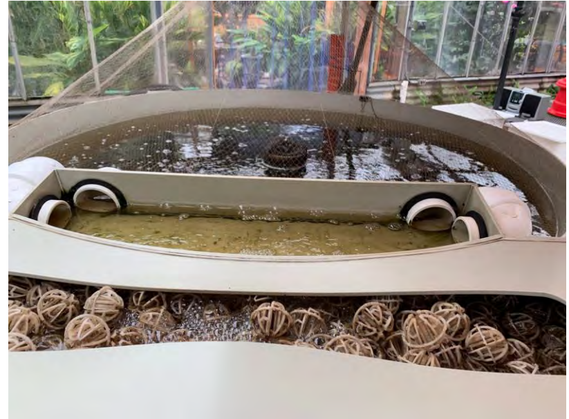
Example of filter media used in a large scale system
