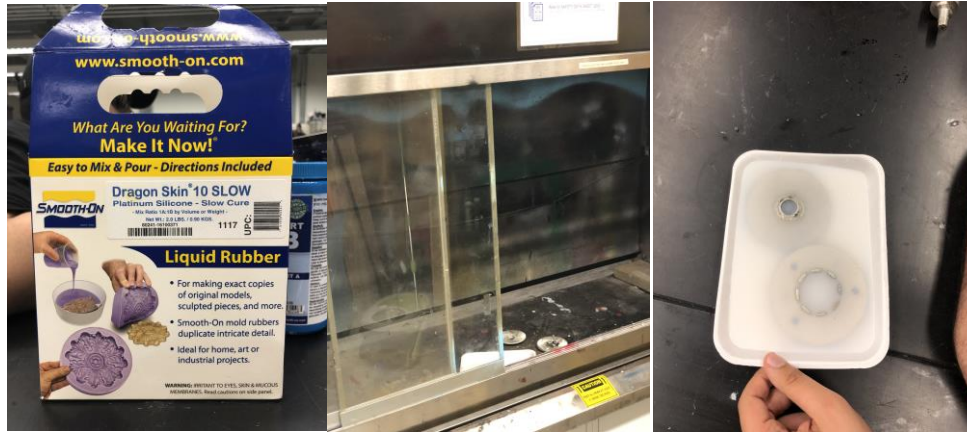
Figure 11 Liquid Rubber being cast onto the plates as plate material.
