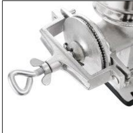
Figure 7: Two plates with sharp teeth made of cast iron with almost no distance between them
