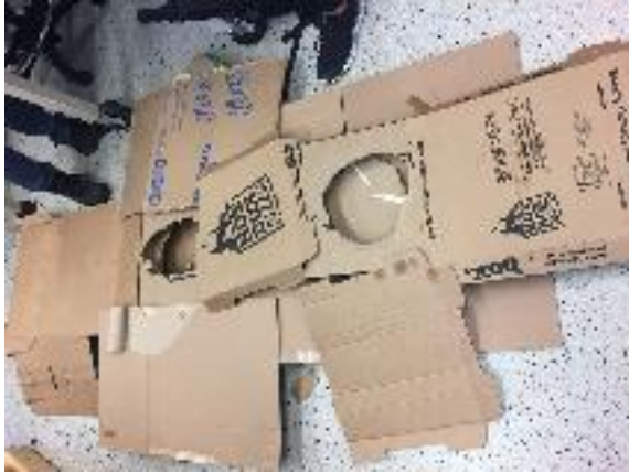
Figure: Artificial pothole; Early prototyping test of Kinect sensor.
