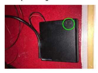
The battery housing supports 4 AA rechargeable batteries. Each cell has a voltage of 1.2V, so total voltage provided is 4.8V to the Arduino. Positive and negative leads are wired through the voltage in male plug. Batteries should be recharged using the provided battery charger.
