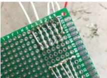
The protoboard houses the resistors and female receptacle for the wire harness. All connections are made on the back through solder points and wire.
