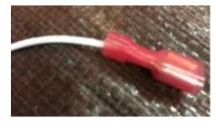
This is the spade terminal that the 5v and normally open pins will connect to on the wire harness. The wires are crimped into the insulated spade terminal and secure to the pinouts on the trigger. Be careful in removing the plug, as the crimped wires are delicate and might back out.
