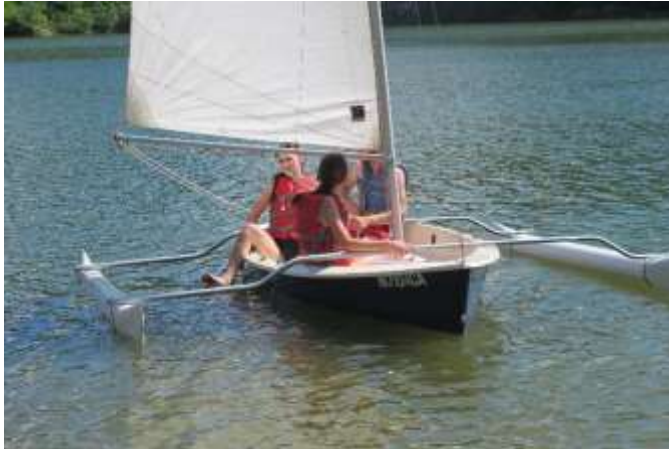
Figure 6.5-1: Prototype outrigger testing while sailing
