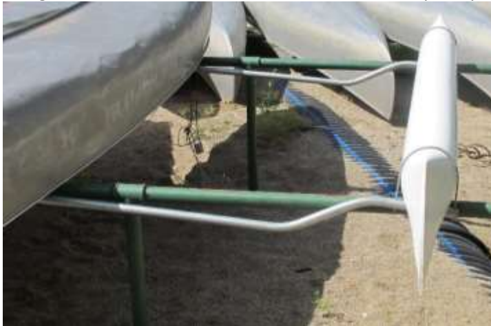
Figure 6.5-3: Canoe outrigger attached to the canoe. It is currently sitting upside down on a rack. The outriggers are not completely circular, but rather more of a petal shape on the edges.
