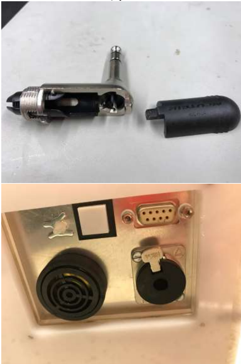
Figure 6 NP3RCS Right Angle Connector
