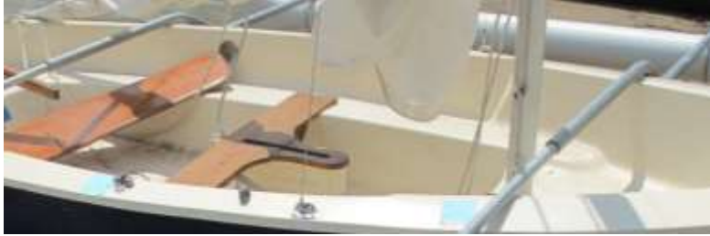
Figure 6.5-4: Interlocking metal bars of outriggers
