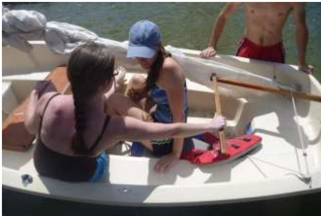
Figure 6.4-8: Trough seating with counselor sitting on boat seat and camper in trough
