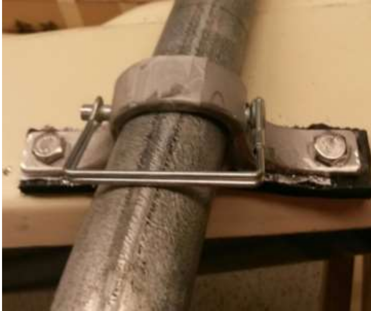
Figure 6.5-6 Picture of clamp that secures the outrigger
